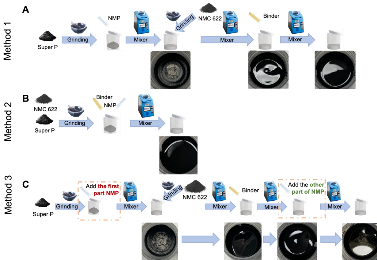
Figure S1. Detailed ink preparation process with optical images of each mixing step for the (A) M1, (B) M2, and (C) M3 inks.
